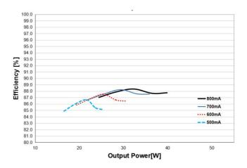
Typical Efficiency vs load of EM FIT 40W 800 CS L G2
