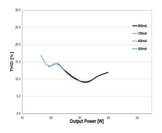
Typical THD vs load of EM FIT 40W 800 CS L G2
