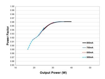
Typical Power factor vs load of EM FIT 40W 800 CS L G2
